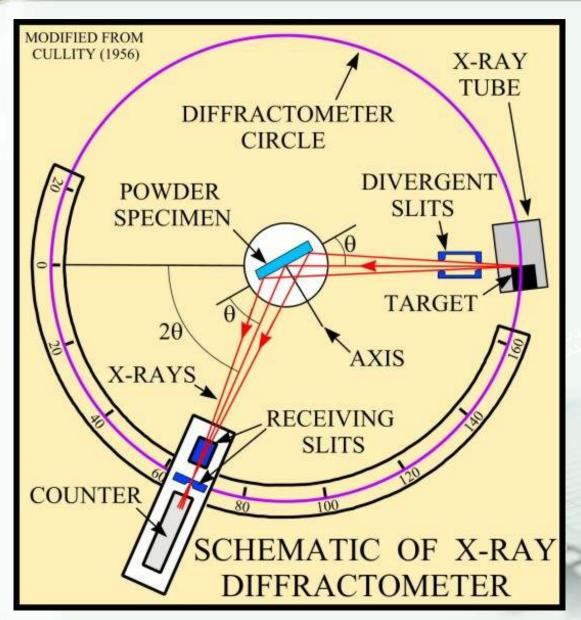
How the Diffractometer Works?
